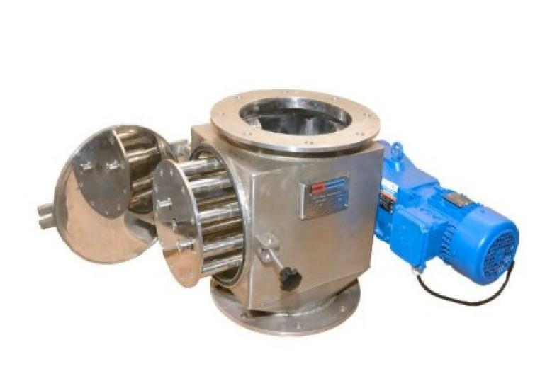
PERMAG's Rotary magnetic separator is an inline magnetic separator used in vertical process lines for the extraction of ferrous particles from difficult to process substances that are prone to bridging or caking.
